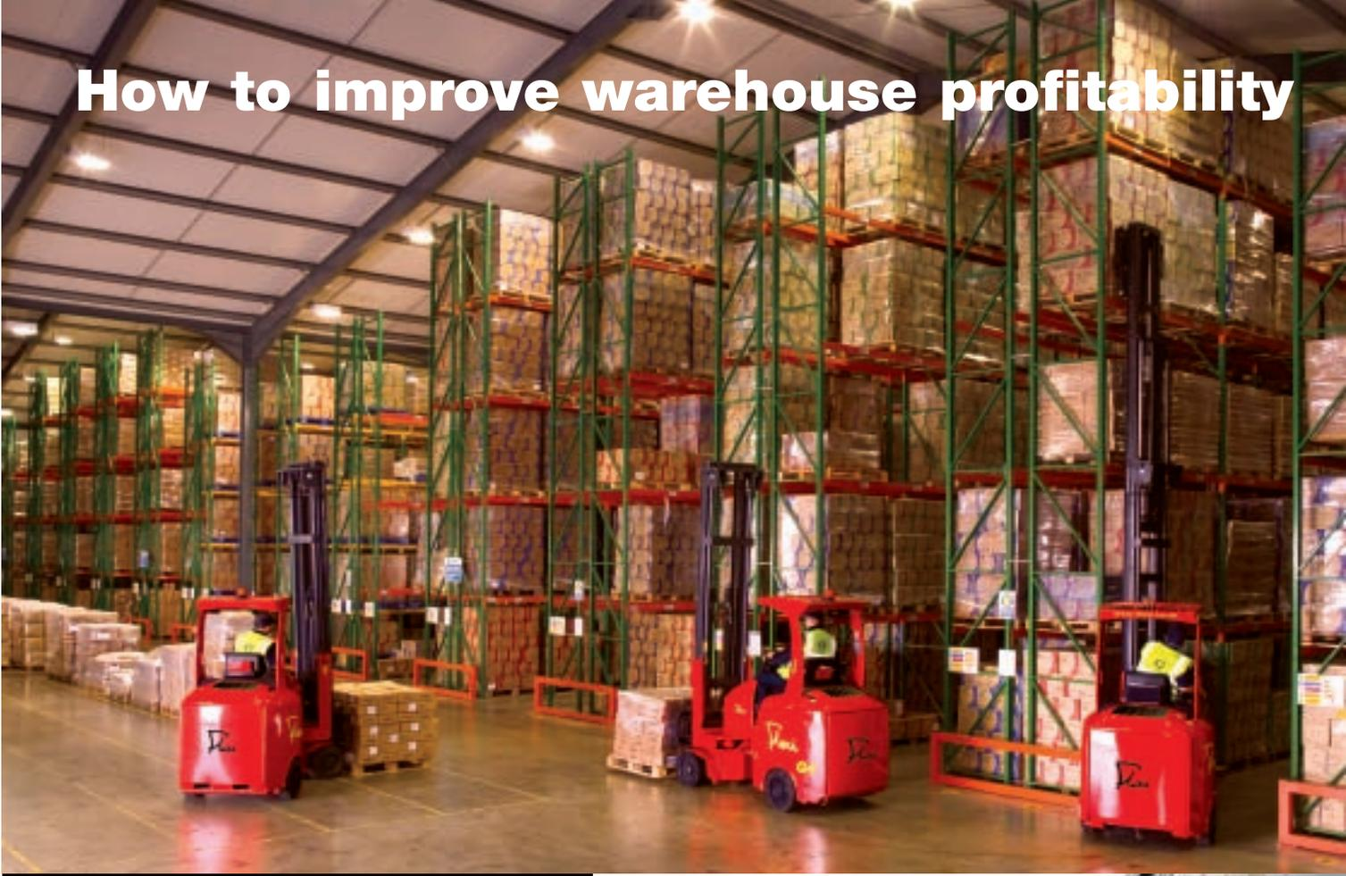
**FLEXI works in just 1642mm (euro)\* or 1762mm (ISO)\* aisle widths - liberating a potential **30% more** warehouse capacity compared with conventional reach trucks.**
