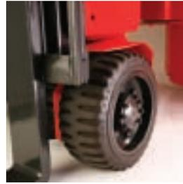
Four large cushion rubber tyres deliver optimum performance and traction in the loading yard. They're also resistant to damage which means a long service life and less downtime.
